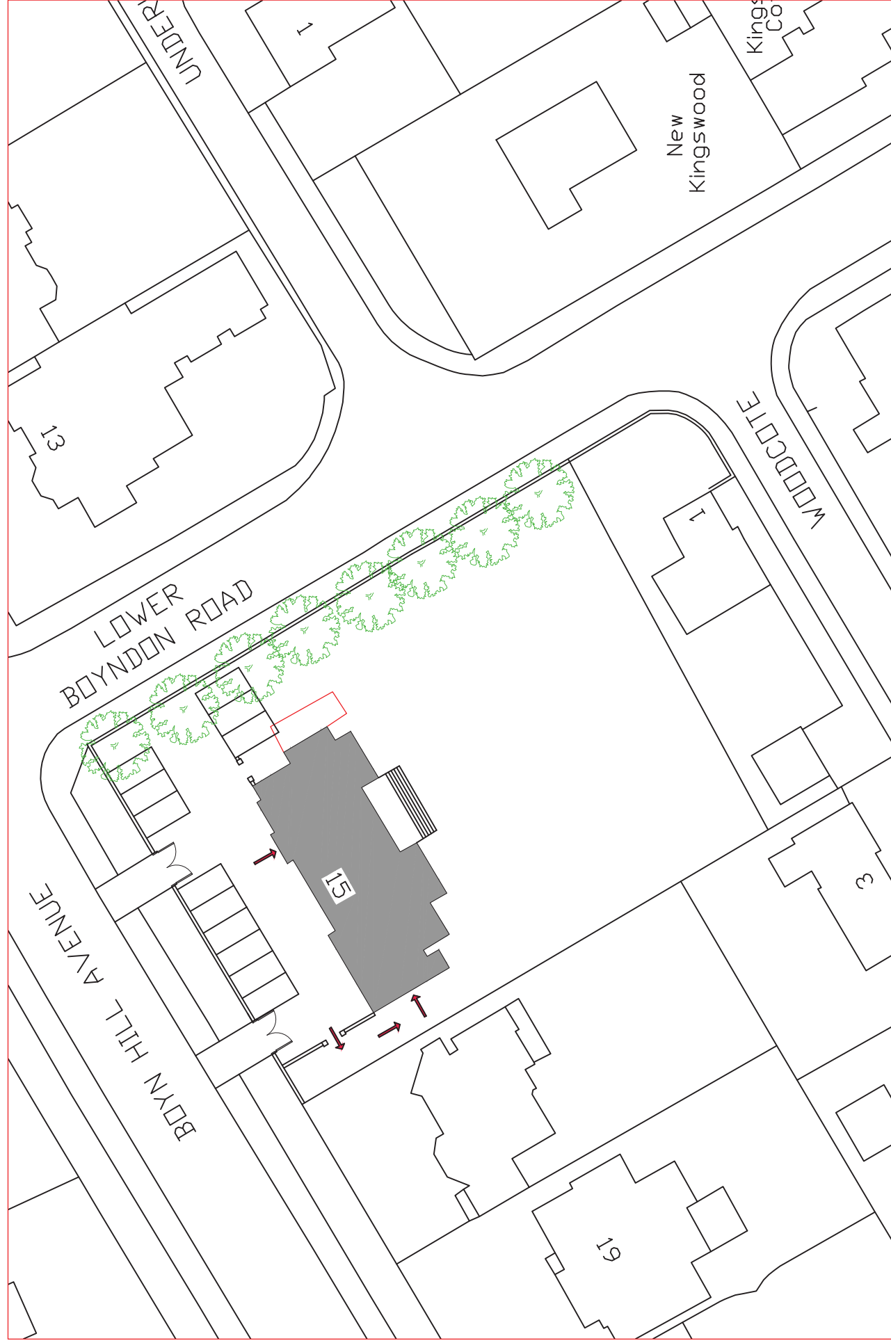
SITE PLAN OPTION 3 - 12 CAR PARKING SPACES - subject to dwarf wall and associated gate post being re-positioned + subject to tree survey and confirmation of parking beneath retained tree. (Copper Beech?)
